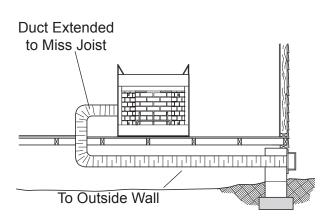
Figure 18 - Installation Above Basement or Crawl Space
